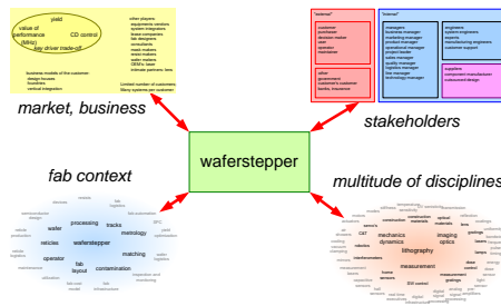
Figure 12: Complexity of Waferstepper Context
