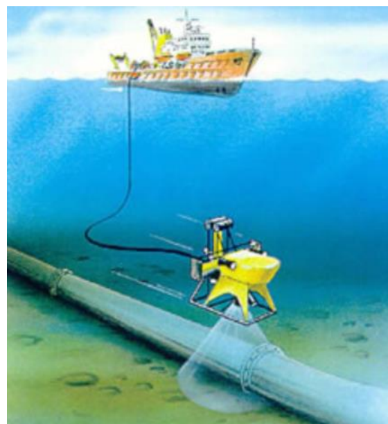
Figure 1. Illustration of a traditional pipeline inspection with MPV and ROV
