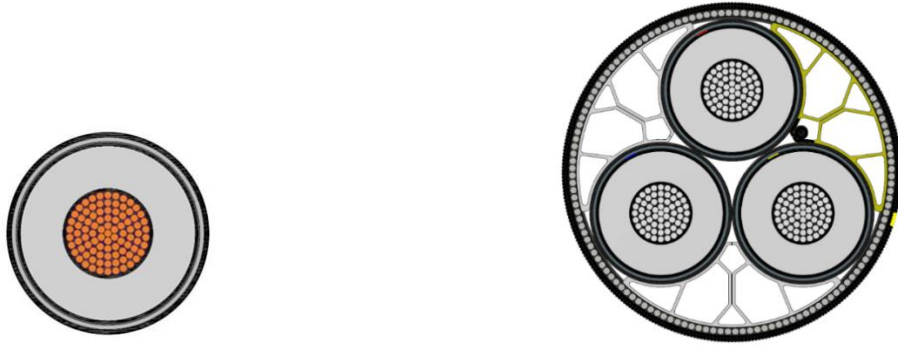
Fig. 4. Cross-section drawings of (a) single-core cable and (b) three-core cable.
