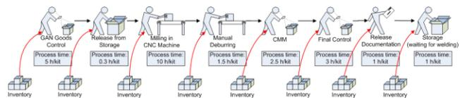
Figure 7. Processing times and intermediate stores for part of the production line
