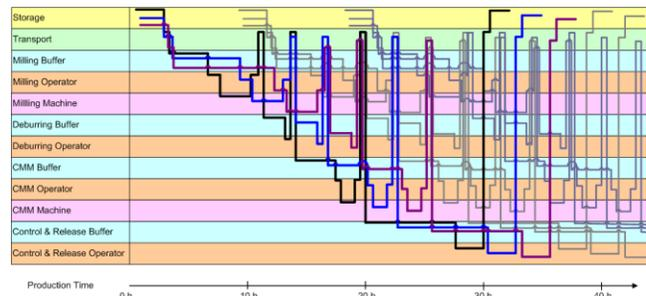
Figure 8. The component workflow in time with swimming lanes per resource
