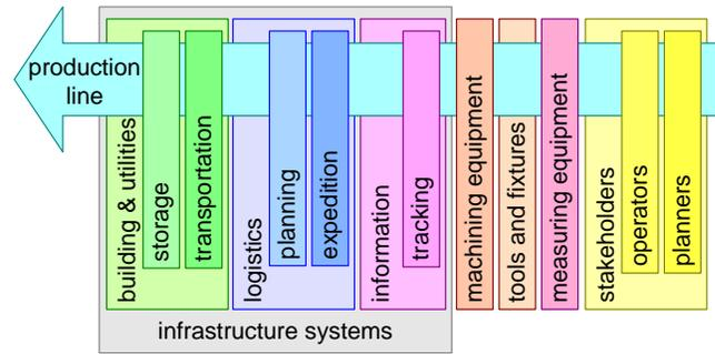
Figure 4. A single production line uses many infrastructure systems and specific systems.
