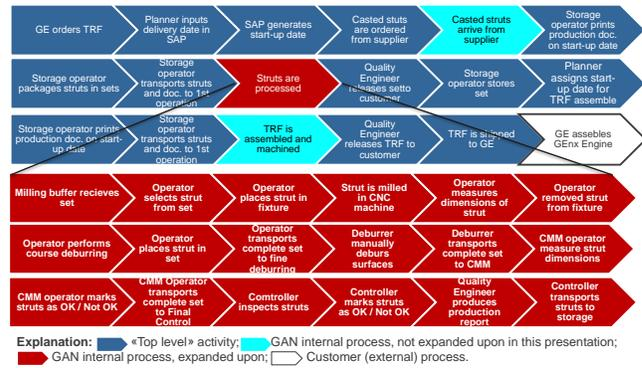
Figure 6. Example model of top-level and component-level workflow process
