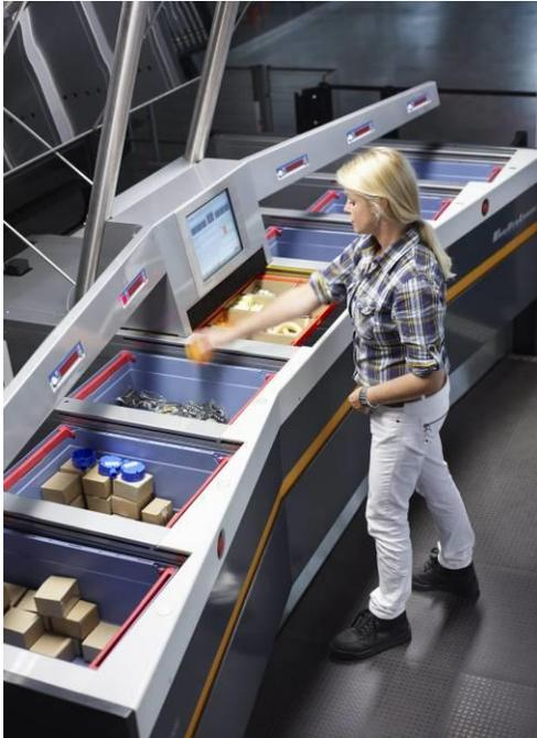
Figure [Photo Pick and Place] An item pick-and-place workstation ([PICK@EASE.4](http://www.vanderlande.com/) from Vanderlande Industries B.V., see <http://www.vanderlande.com/>). Totes at the left and the right with the small displays on top contain orders; the tote in the middle with the large display contains the stock items.
